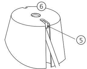
⑥ The luminaire head becomes hot in the area of the LED during operation. The LED must not be touched or cleaned directly (mechanical / chemical / electrostatic damage to the LED).
