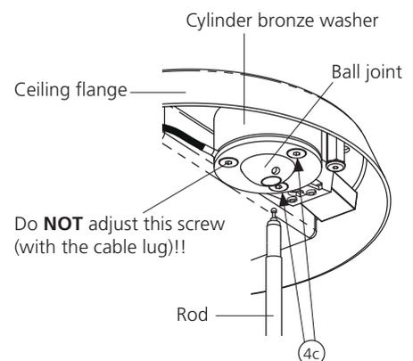
**Loosen or tighten these 2 screws accordingly.**
