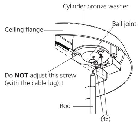
Loosen or tighten these 2 screws accordingly.
